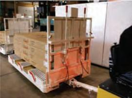
Optimal Steer Manual Transfer Cart with Conveyor Brake & Manual Stop Levers Ref: CT72
