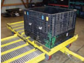
Optimal Steer Double 48x45 Box Manual Transfer & Lift Gate Cart Ref: CT78
