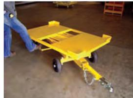
Optimal Steer Manual Rotate Deck with 180° Detent Ref: CT73
